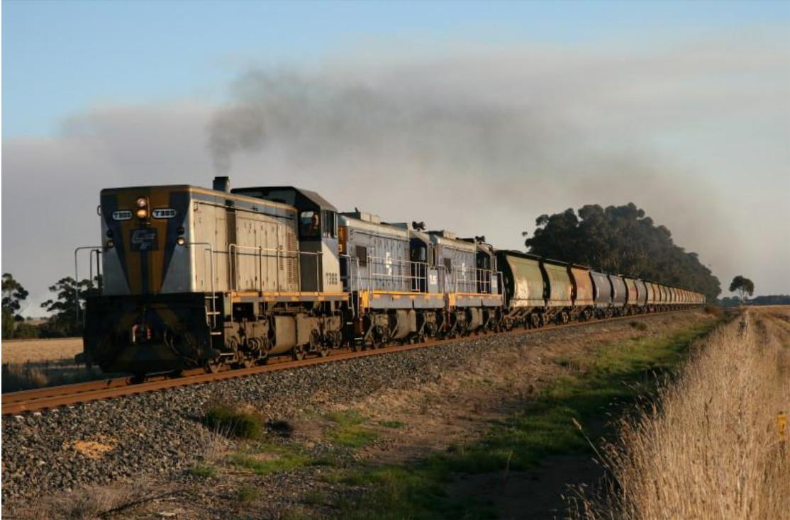
Hired from CFCLA were T385, TL155 and TL153, seen here approaching Ararat with empty hoppers after discharging at Geelong on 7th April. The TL's were built by Clyde in 1955 and 1957 for the Kowloon - Canton Railway, and have recently been returned to Australia. They are based largely on Victoria's flat top T class locos. Interestingly, Austrains will be bringing out a model of the K&C Railways 51 class as they were known in Hong Kong.
